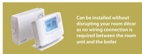
The wireless room thermostat HCW80 sends heat demand signals (RF 868.3 MHz) to the relay module HC60NG. It can be used to control gas and oil boilers, a variety of valves and actuators, or electrical heating systems.
